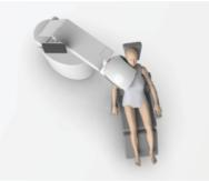
The proposed QT Orthopedic Scanner being applied to shoulder imaging Image 12
